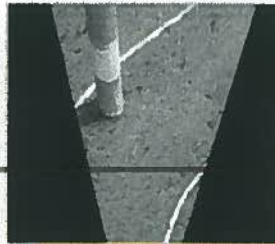
Figure 14. Converted color space, smoothed and warped for perspective.
