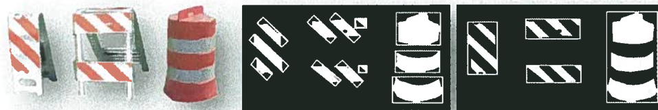
Figure 12. Conceptual example of blob detection and blob merging of complex
