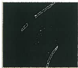
Figure 18. Edge detection with barrel obstacle removed, some noise remains.
