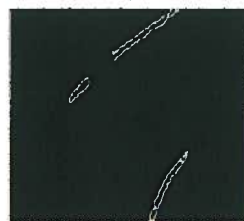
Figure 17. Removal of noise through small blob finding.
